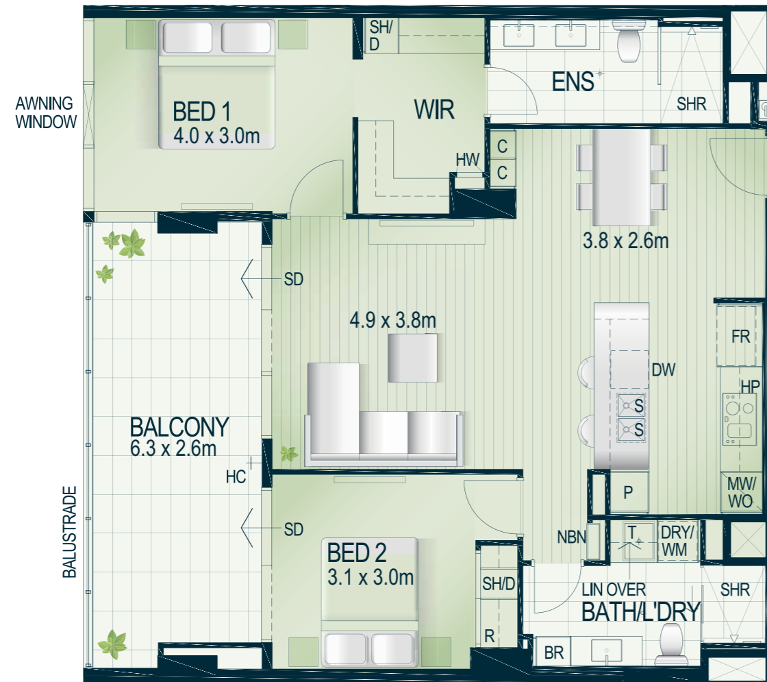
UNIT PLAN ABOVE IS TYPICAL. REFER TO OVERALL PLANS FOR LOCATION, ORIENTATION, VARIATIONS & BALCONY DESIGN.
